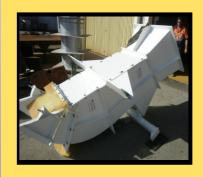
Finally the item is sandblasted externally and repainted. Identification numbers are reapplied prior to shipment back to the client.
